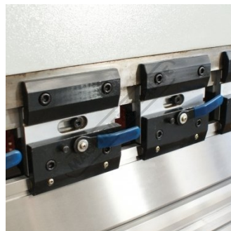
Quick Action Intermediate Clamps
