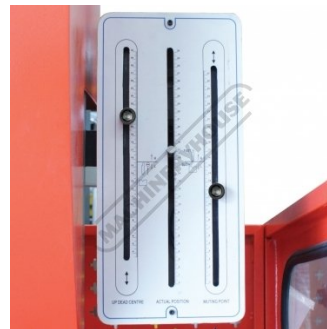
Adjustable Travel Limit Control
