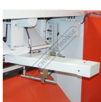
Motorised Backgauge Close Up
