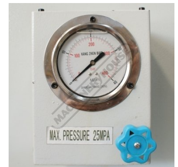
Adjustable Pressure Control
