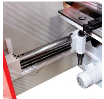
Estun NC E21 Control Ballscrew Backgauge
