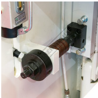
Quick Action Blade Clearance Adjustment
