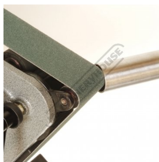
Internal Pipe Chamfering
