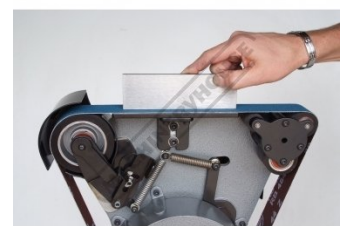
Flat Grinding on Platen
