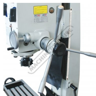
Fine Feed Handwheel Operating Quill Feed
