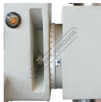
Tilting head to 90 Degrees from vertical
