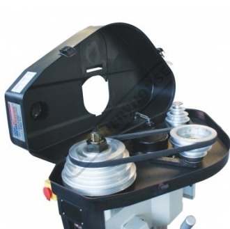
Belt Drive 12 speeds 100 2080rpm Left View
