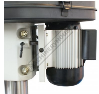
Motor Belt Tension Adjustment
