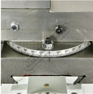
Compound Slide Angle Scale
