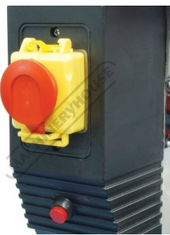
Emergency Stop Switch and Light Switch
