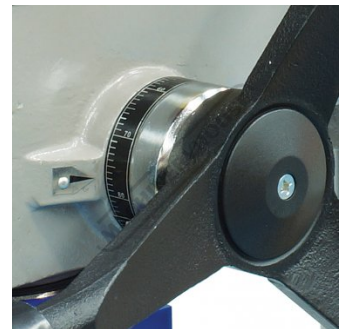
Drilling Depth Stop Setting With Scale
