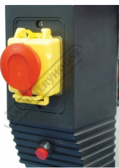
Emergency Stop Switch and Light Switch
