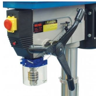
1 Piece Cast Iron Drilling Lever
