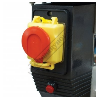
Emergency Stop Emergency Switch and Light Switch
