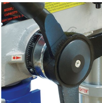
Drilling Depth Stop Setting With Scale
