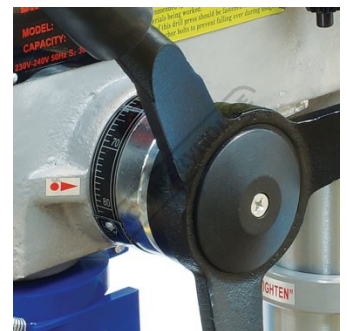
Drilling Depth Stop Setting With Scale
