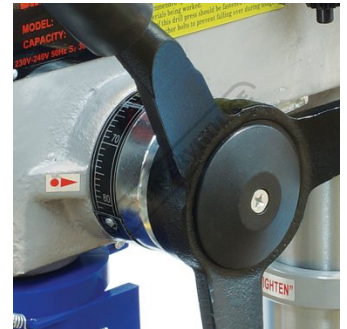
Drilling Depth Stop Setting With Scale
