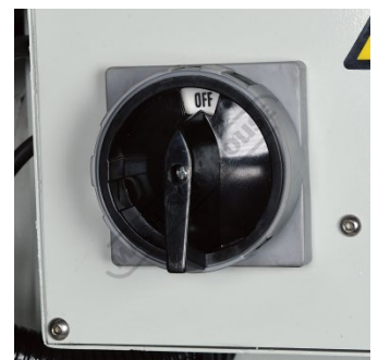
Main Isolation Switch
