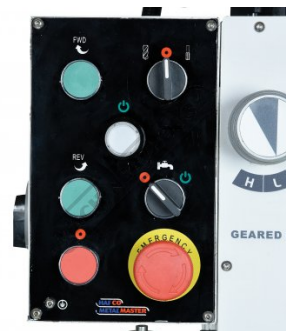
Control Panel with Tapping Function
