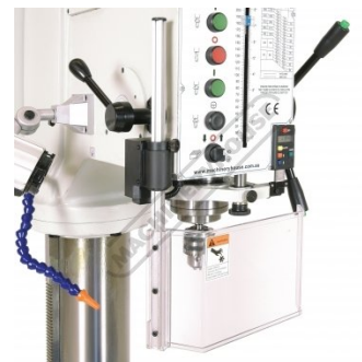
Interlocked Spindle Safety Guard
