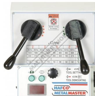
Drill Speed Selection Levers & Speed Chart
