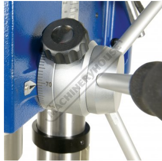
Drilling Depth Stop Setting With Scale
