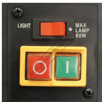
Magnetic Switch and Light Switch
