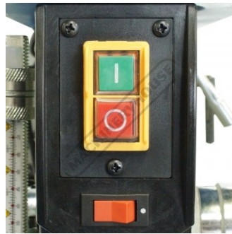
Magnetic Switch and Light Switch
