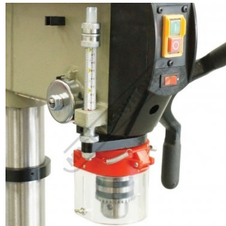
Drilling Depth Stop Setting with Scale
