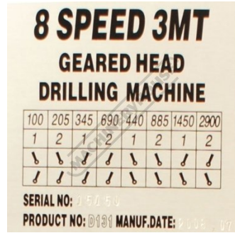
8 Drilling Speeds From 100 2900rpm
