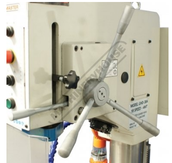
Adjustable accurate depth setting with auto feed out for increased productivity
