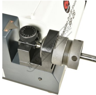
Drill Setting Gauge Shown with 13mm Drill
