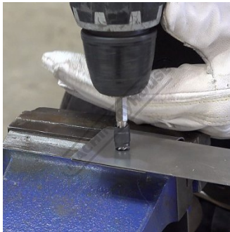
Push Down Ready For Drilling
