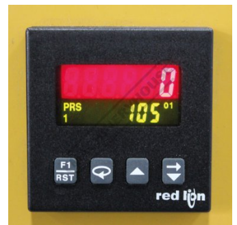
Digital Degree Display with Auto Stop Programming
