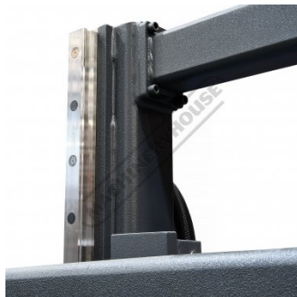
Linear Guide Ways on Posts
