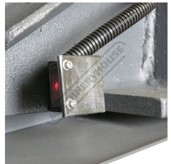
Auto Optical Material Height Adjustment
