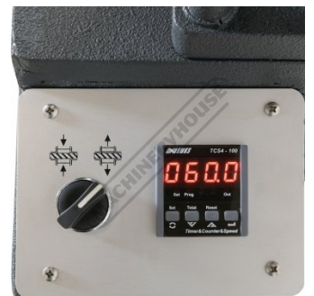
Head Lock Switch With Digital Mitre Angle
