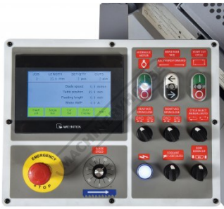
Touch Screen Controller
