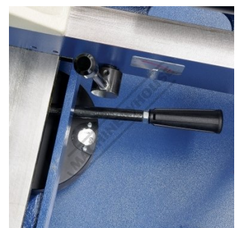
Swivel Head Locking Lever with Magnified Scale
