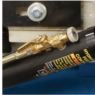
Hydraulic Ram Down Feed Control
