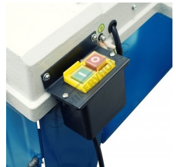
Main Power Switch
