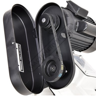
3 Speed Pulley Drive System
