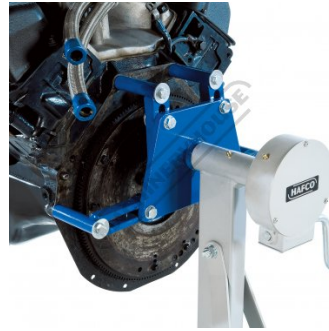
Mounting Positions On Engine
